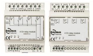
The VMB4RYLD is a 4-channel voltage-out relay module with common neutral poles, where only the live pole is switched on each channel. The live and neutral wires, normally coming from an isolated and protected circuit breaker, are simply connected to the input contacts of this module, which makes them available as 4 relay outputs.
