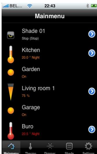
Home center for iPhone lets you operate and monitor all controls of your system. On connection, all available controls are downloaded to your iPhone. Each control can be operated by tapping it. The result of your action will immediately be visible in your house (for instance light goes on) and in the iPhone app (icon will be lit).
