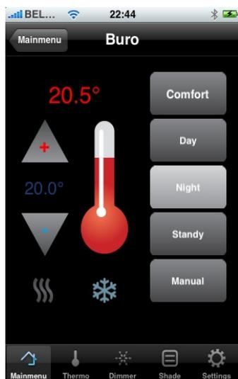
In the list, thermostat are displayed as an item with a thermometer and its name next to it. You can also read the current temperature and the active regime.
